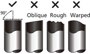
**DO NOT DEFORM PIPE WHILE CUTTING**
