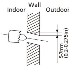
**NOTE:** When the gas side connective pipe is  $\Phi$  16mm(5/8in) or more, the wall hole should be 90mm(3.54in).
