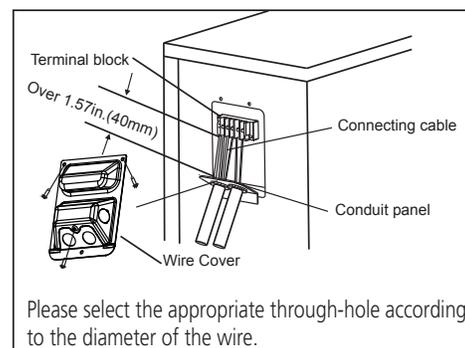
Please select the appropriate through-hole according to the diameter of the wire.
