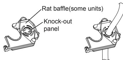
**NOTE:** If the size of the cable is too big, remove the middle small plastic knock-out panel to create a slot through which the cable can exit. If you want to remove the chassis or drain hose, please remove the rat baffle first.
