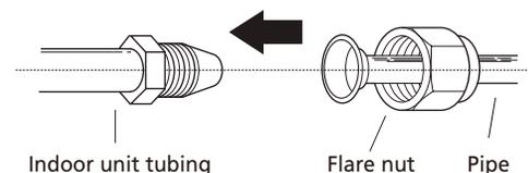
2. Tighten the flare nut as tightly as possible by hand.
