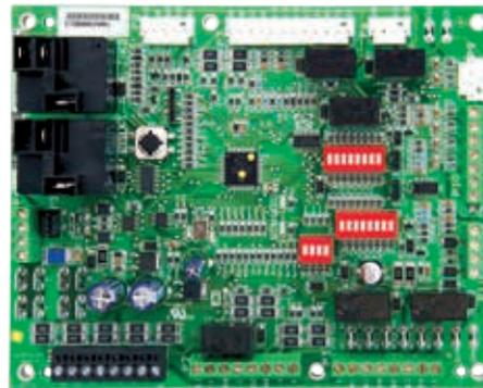
Locate the version level of the DXM2 board and thermostat or service tool on the screen. You can locate the part number on the board and compare it to the table below.
