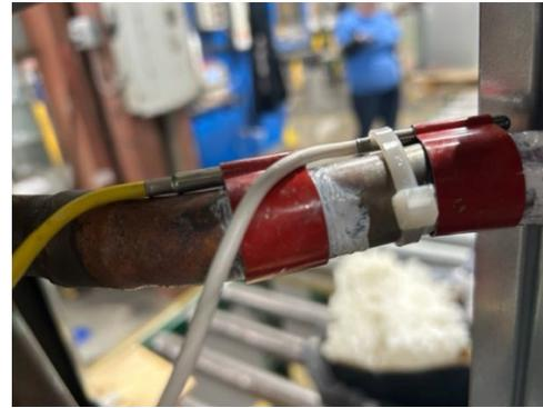
(Black) Compressor Discharge Temperature (CDT) sensor
