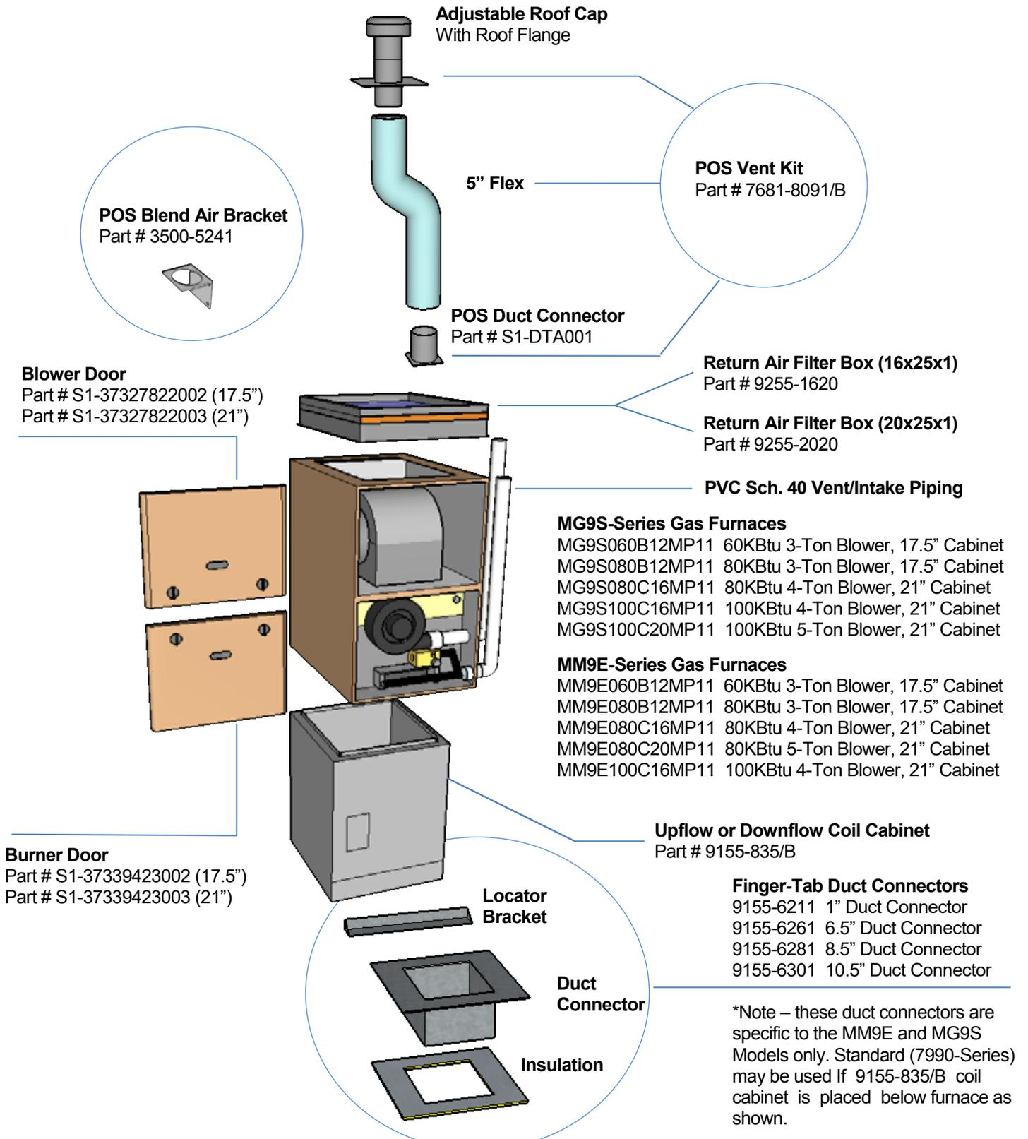
MG9S/MM9E-Series 95% Gas Furnace, converted to *Up-Flow on Fabricated Shelf*
