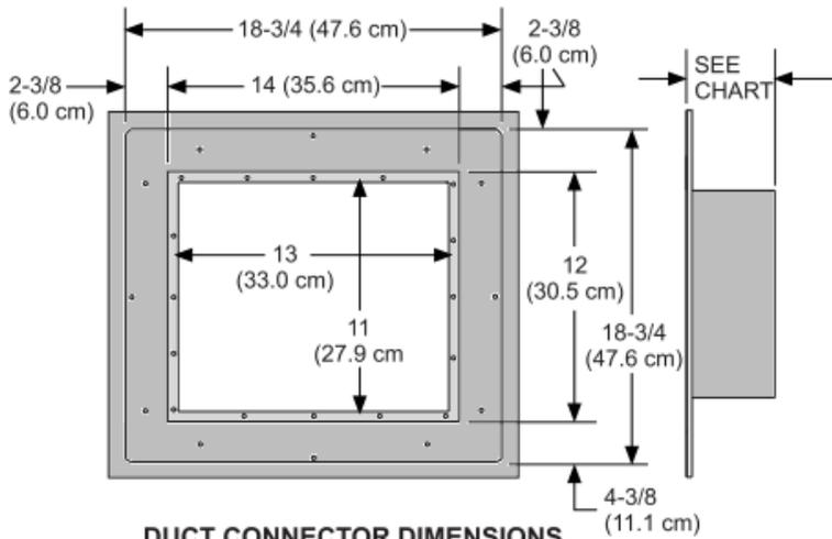
**Screw-Tab Duct Connectors**
