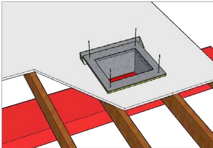
**Step 4:** Furnace is slid back to against locator plate and secured to floor using methods detailed in install manual.
