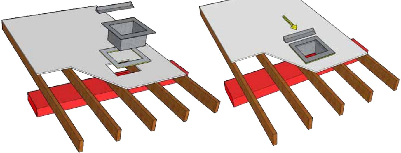
**Step 3:** Duct connector is then attached to the floor using appropriate screws, flat-head nails, or staples.
