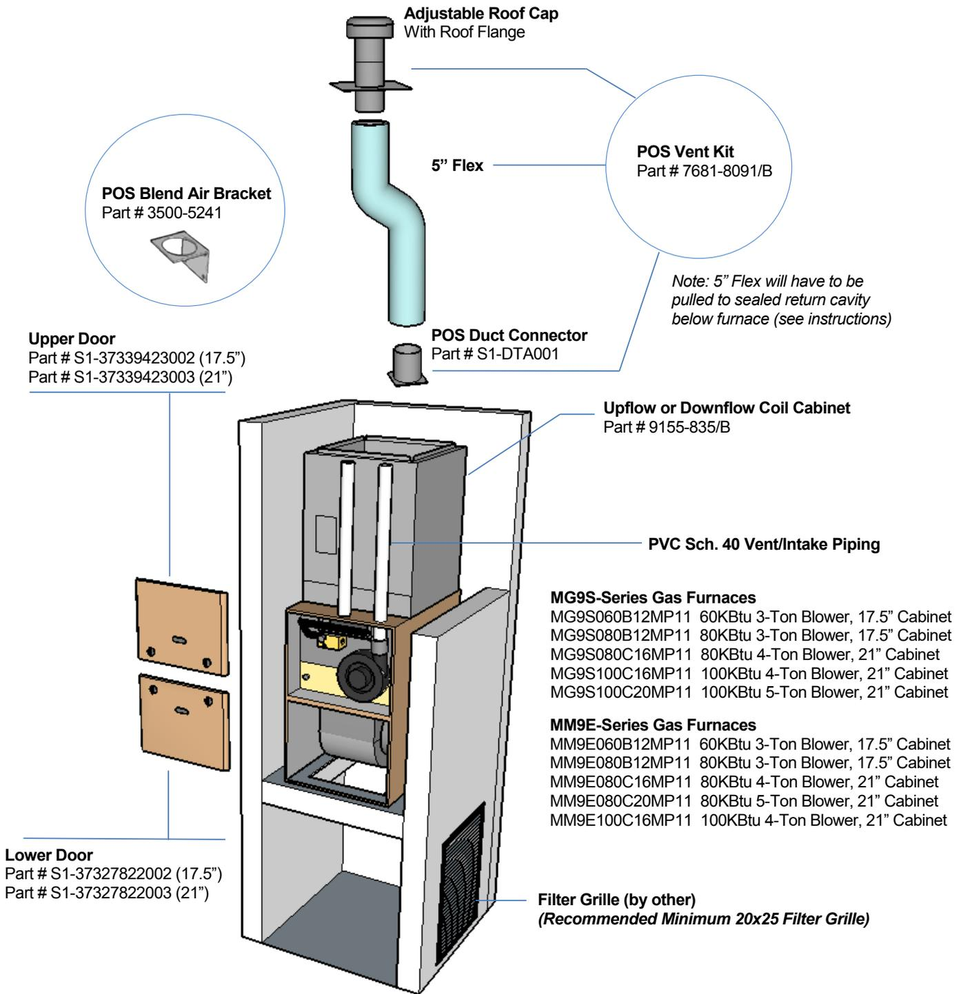
MG9S-Series 95% Gas Furnace converted to *Up-Flow with Side Return*
