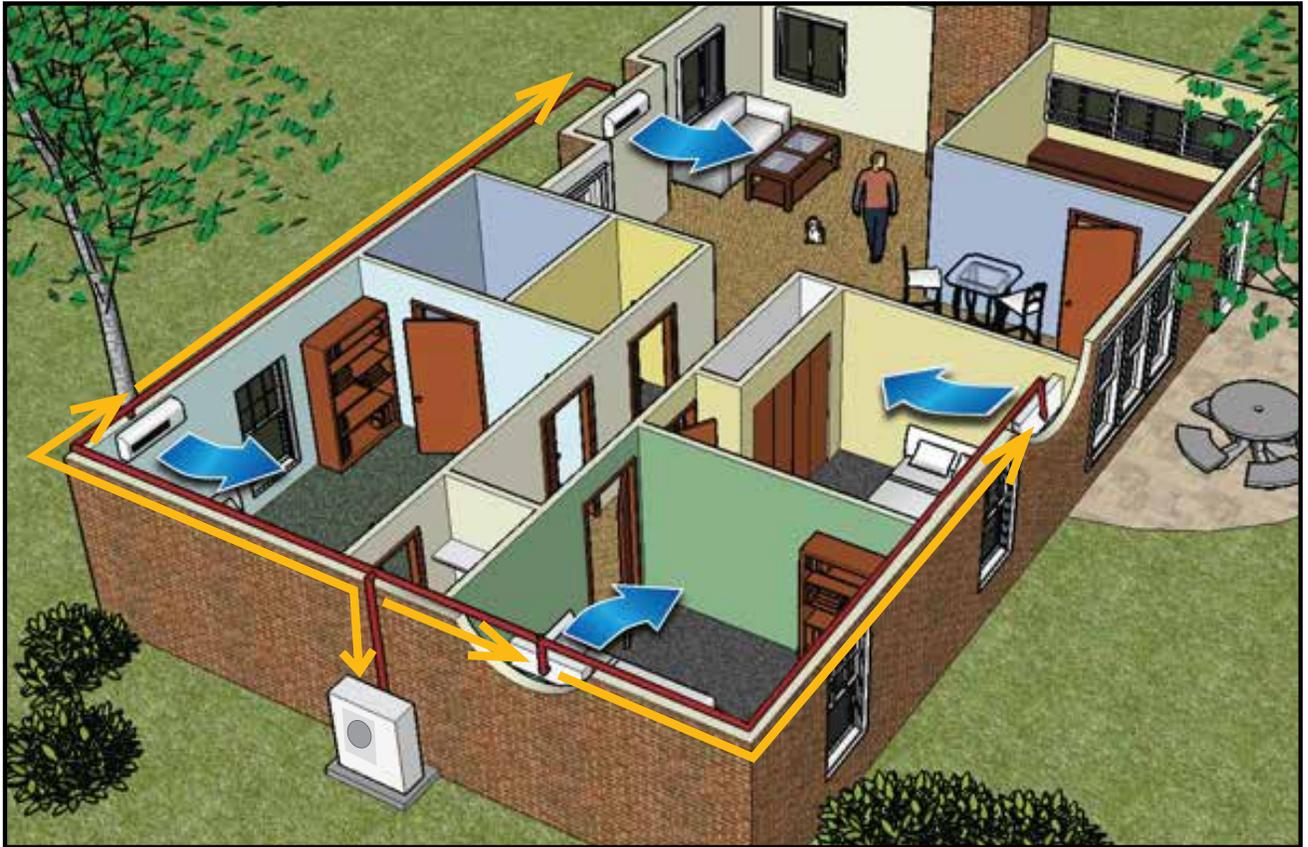
You can see how one outdoor condenser is used in conjunction with multiple indoor air handlers in a single structure. Air handlers can be installed up to 115' (depending on model) from the condenser, so you can place the condenser in the best location for your landscaping.
