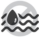
DO NOT install the indoor unit in a moist environment. Excessive moisture can corrode the equipment, electrical components, and cause electrical shorts.
