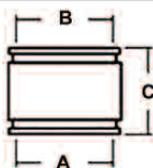
**Note:** Tighten bolts to 60 inch lbs. min. / max torque. Tested to maintain 4.3 p.s.i. maximum line pressure (10' head pressure) Tested and Certified to ASTM Standard 1173-2010.
