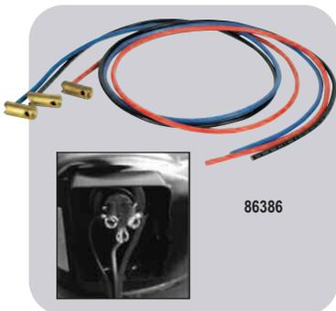
The MARS Term-Lok is a brass cylindrical tube with a diameter large enough to slip over the pins and has a stainless set screw to lock onto the terminal. Term-Lok comes in packages of one or three terminal locks with color coded 65 strands, 600 volt permanently attached wire, with wrench provided for easy application. Once installed the compressor cover may be placed back over the terminals without any obstructions.
